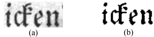
Figure 2. (a) Original image and (b) the corresponding binary image after adaptive binarization
