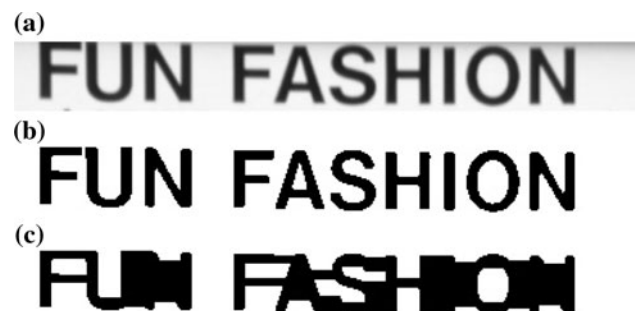
Fig. 14 Word segmentation. a Grayscale image, b binarized image, c RLSA result
