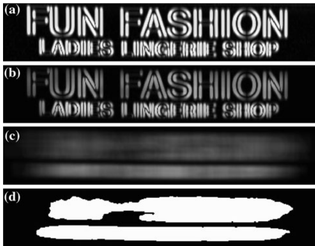
Fig. 11 Text line localization. a Sobel gradient, b gradient after multiplying with saliency map, c gradient after Gaussian smoothing, d gradient after Otsu thresholding
