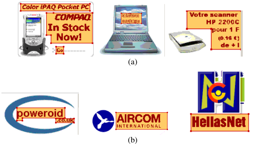
Fig. 5. Example of the ground truth text annotations: (a) From the laptop offers domain (b) from the job offers domain.
