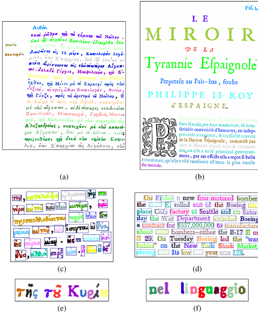
Fig. 13. Text line, word and character segmentation examples extracted by the propose method: (a) text line segmentation example of Greek historical document, (b) text line segmentation example of French historical document, (c) word segmentation example of Greek historical document, (d) word segmentation example of English historical document, (e) character segmentation example of Greek historical document and (f) character segmentation example of Roman historical document.
