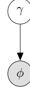
Fig. 1. A generic view of the proposed graphical model. \gamma stands for the word transcription to be estimated and \phi stands for the observed PHOC vector. We aim to find the most probable transcription \gamma for the given encoding \phi .
