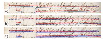
Fig. 4. Baseline sets of four GT baselines (blue) and hypothesis (HY) baselines (red) in a). The normalized polygonal chains in b) (for illustration purposes, every  $25^{\rm th}$  vertex is displayed). GT baselines with tolerance area estimated in c) (here,  $t_g$  is roughly  $20 \mathrm{px}$ ).
