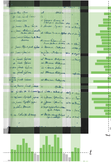
Fig. 3. Document image with the corresponding SIFT features. The SIFT features are binned with 50 column and row wise and the rows and columns below a certain threshold (1/3 of the maximal value) are skipped. Then the area of the remaining rows and columns is calculated, which is the estimated area for the writing zone.
