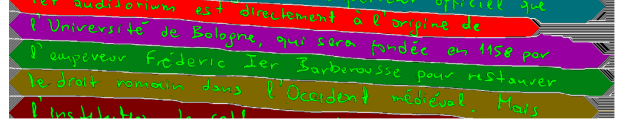
Figure 5. Part of an indicative LLA(x,y) with l(x,y) superimposed as bright green. White pixels have the null label, black pixels were filtered out and colored pixels represent different line areas.
