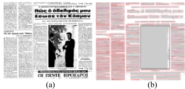
Fig. 2. (a) Original image, (b) Image IDR with all segments defined using Connected Component Analysis.
