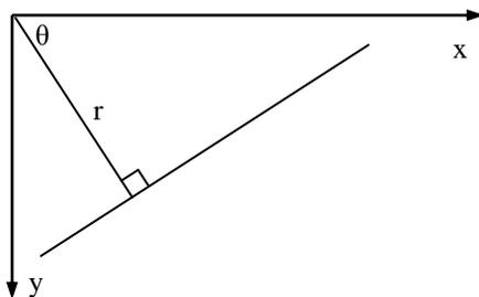
Figure 6: Parametrization of a straight line for application of Hough transform.
