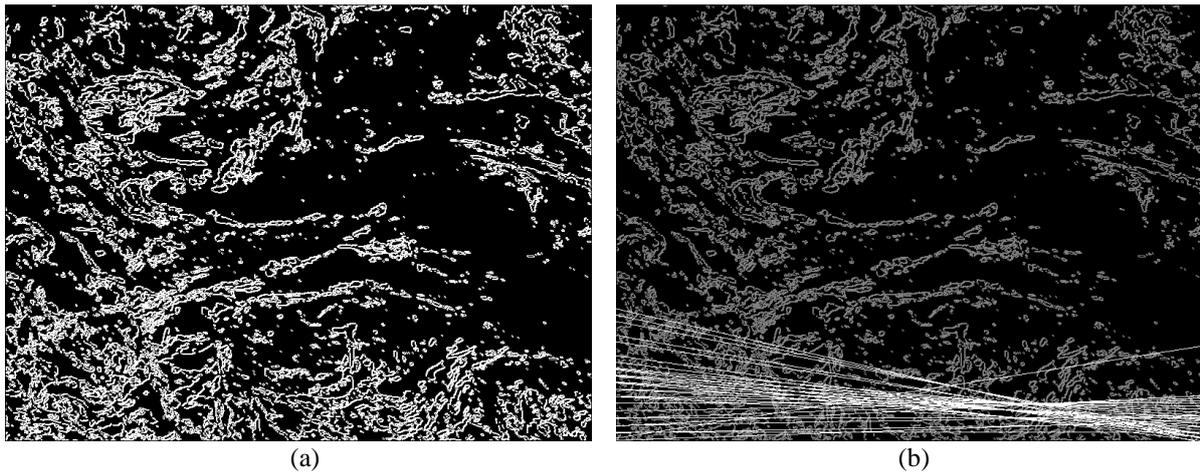
Figure 10: (a) Binary image produced by extracting the edges of Figure 8b, and (b) the most prominent lines found by the original Hough transform.
