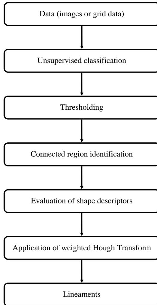
Figure 1: Outline of the procedure for the delineation of lineaments.
