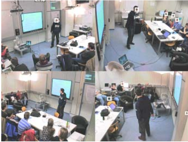
Figure 2. Frame-level face detection result on synchronized images from the four available camera views, using the FloatBoost frontal and side face detectors.
