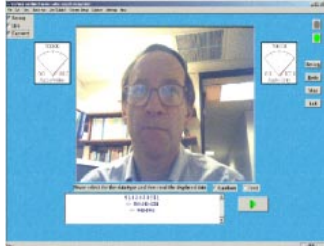
Fig. 5. The prototype graphical user interface. Two central windows depict the captured video and uttered vs. recognized text, while two meters show the resulting audio-only vs. audio-visual word error rates.
