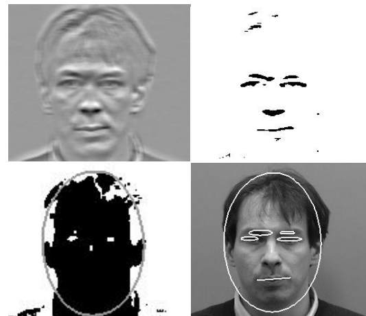
Figure 3: Examples of processing steps to identify facial features. The top row shows two steps of the shape analysis - left: after bandpass filtering; right: after thresholding. The bottom left image shows the result of the color segmentation. The bottom right displays the result.
