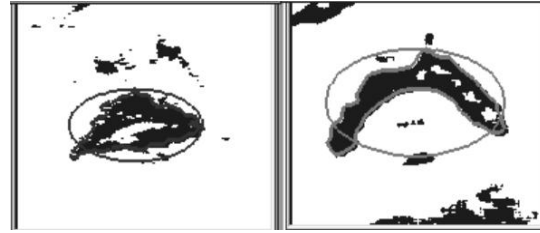
Figure 6: Color segmentation of the mouth area. The left image shows areas with a hue of the lips, the right image indicates hue of the moustache.
