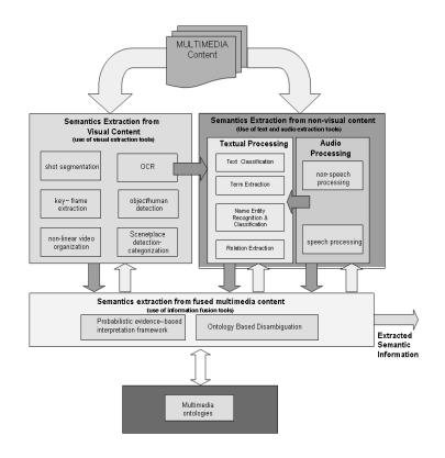
Figure 2 Architecture of the semantics extraction subsystem
