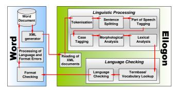
Figure 4: The architecture of the SCHEMATOPOIESIS controlled language checker. *Ellogon* was used as a "vehicle" for embedding the checker under Word. Communication between Word and *Ellogon* was achieved by means of XML and DDE messages.
