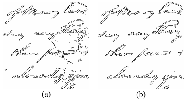
Figure 4. Example of edge images: (a) edge map I_E of the original grey scale image I_F of Fig. 3(a) after applying the Canny edge detector and (b) adapted edge map I'_E containing only those connected components of I_E that have a significant overlap with the binary image B_R of Fig. 3(e).
