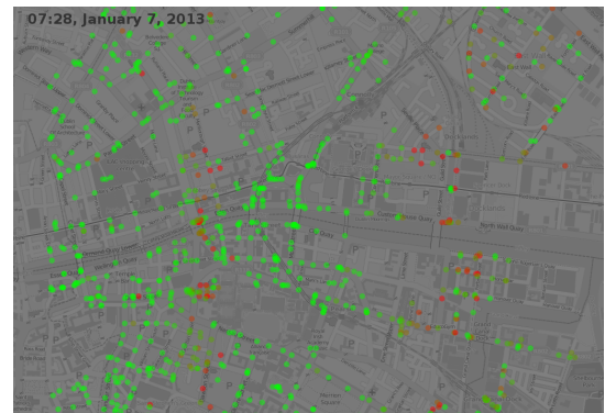
Figure 9: Traffic Flow estimates obtained by Gaussian Process Regression. Green dots correspond to low traffic whereas red dots indicate congested locations.
