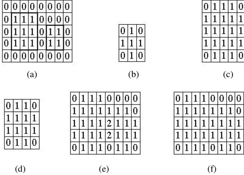
Fig. 3. (a) Original image consisting of two rectangular blocks  $A_1$  and  $A_2$ . (b) Structuring element  $B$ . (c), (d) Dilation of two blocks. (e) Final image after replacing the blocks by their lookup tables. (f) Final dilated image.
