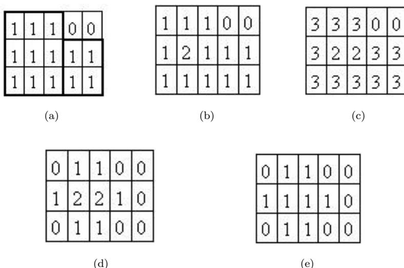
Fig. 6. (a) Original image consisting of two rectangular blocks  $A_1$  and  $A_2$ . (b) Resulting image after applying Step 1 of the opening algorithm described in Sec. 3.4. (c) Resulting image after applying Step 2 of the opening algorithm described in Sec. 3.4. (d) Image after the dilation of Step 3 of Sec. 3.4. (e) Final opened image.
