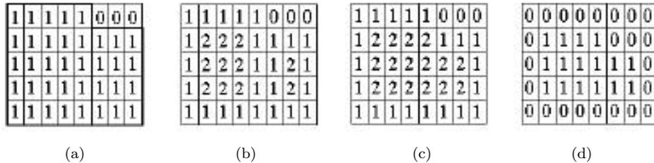
Fig. 4. (a) Original image consisting of two rectangular blocks  $A_1$ ,  $A_2$ . (b) Resulting image after applying Step 3 of the erosion algorithm described in Sec. 3.2. (c) Final image after applying Step 4 of the erosion algorithm described in Sec. 3.2. (d) Final eroded image.
