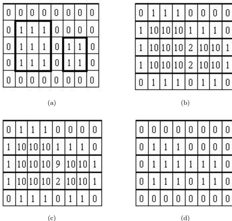
Fig. 5. (a) Original image consisting of rectangular blocks  $A_1$  and  $A_2$ . (b) Resulting image after applying Step 3 of the closing algorithms described in Sec. 3.3. (c) Final image after applying Step 4 of the closing algorithm described in Sec. 3.3. (d) Final closed image.
