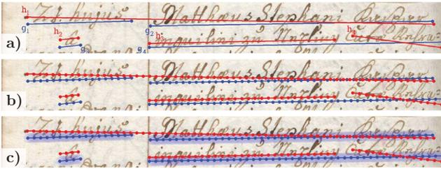
Fig. 4. Baseline sets of four GT baselines (blue) and hypothesis (HY) baselines (red) in a). The normalized polygonal chains in b) (for illustration purposes, every 25<sup>th</sup> vertex is displayed). GT baselines with tolerance area estimated in c) (here,  $t_g$  is roughly 20px).
