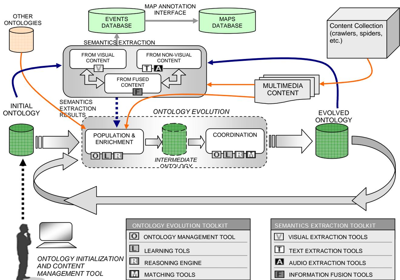
Figure 1. Architecture of the integrated system
