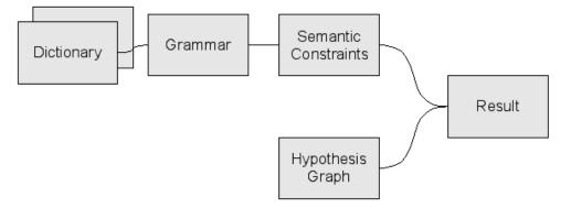
Figure 10. Language models based on finite state transducers can be composed modularly from dictionaries, *n*-grams, grammatical patterns, and semantic patterns. This allows OCRopus to be retargeted and adapted quickly to new document types and languages.
