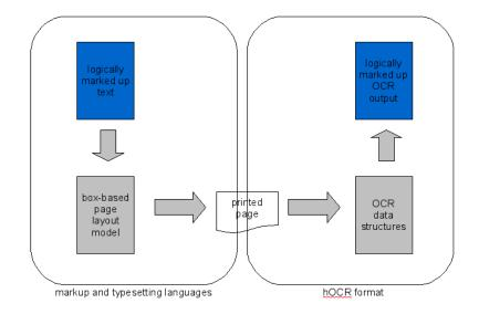
Figure 12. The hOCR format<sup>25</sup> is based on a typesetting model of document generation: documents are generated by flowing logically marked up text into page models consisting of boxes; the hOCR format achieves OCR engine independence by representing these typesetting concepts directly.
