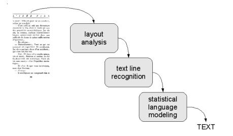
Figure 1. A rough flow diagram of the OCRopus system. The system is strictly feed-forward and consists of three major components: layout analysis, text line recognition, and statistical language modeling. (In addition, it also contains tools for preprocessing and classifier combination.)
