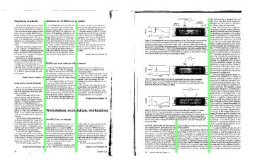
Figure 3. Example of column finding. The whitespace between the columns is identified as maximum area whitespace rectangles with a high aspect ratio and large numbers of adjacent, character-sized connected components.
