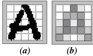
**Figure 3.** (a) The normalized character image, (b) Features based on zones. Darker squares indicate higher density of character pixels.
