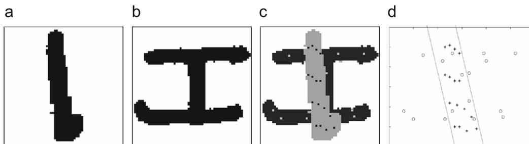
**Fig. 6.** (a), (b) Characters 't' and 'l'. (c) Features at granularity level 2. (d) Representation in feature space: (\*) for 't' and (o) for 'l'. At this level such characters can be distinguished.
