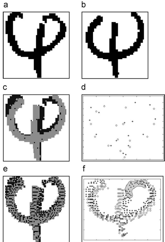
**Fig. 7.** (a), (b) Characters 'φ' and 'ψ'. (c), (e) Features at granularity levels 2 and 4, respectively. (d) Representation in feature space at level 2: (\*) for 'φ' and (o) for 'ψ'. At this level such characters cannot be distinguished sufficiently. (f) Representation in feature space at level 4: (\*) for 'φ' and (o) for 'ψ'. Level 4 works fine for these characters mainly because of the features in the gray region.
