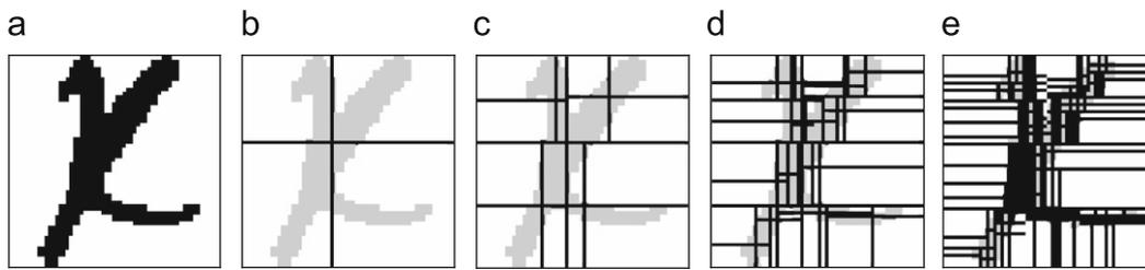
Fig. 3. Character image and sub-images based on DP: (a) original image, (b), (c), (d) and (e) subdivisions at levels 0, 1, 2 and 3, respectively.
