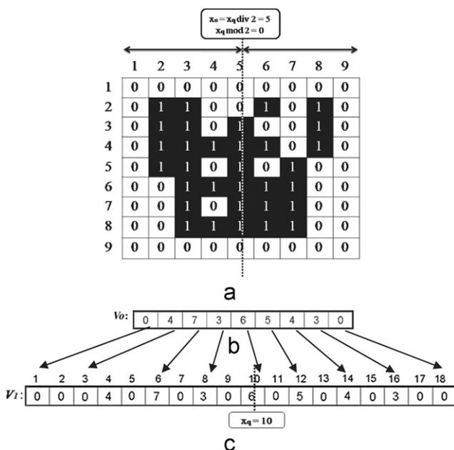
Fig. 1. (a) Example of a vertical division of an image array ( $x_{max}=9, y_{max}=9$ ); (b) vertical projection ( $V_0$ ) and (c) creation of  $V_1$  array from  $V_0$  and calculation of  $x_q$ .
