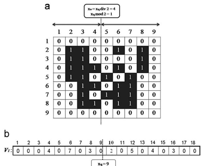
Fig. 2. Example of a vertical division of an image array when  $x_q \bmod 2=1$ .
