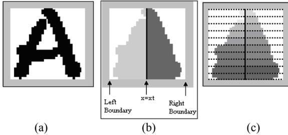
**Fig. 4: Feature extraction of a character image based on left and right character profile projections. (a) The normalized character image. (b) Left and right character profiles; (c) The extracted features. Darker squares indicate higher density of zone pixels.**
