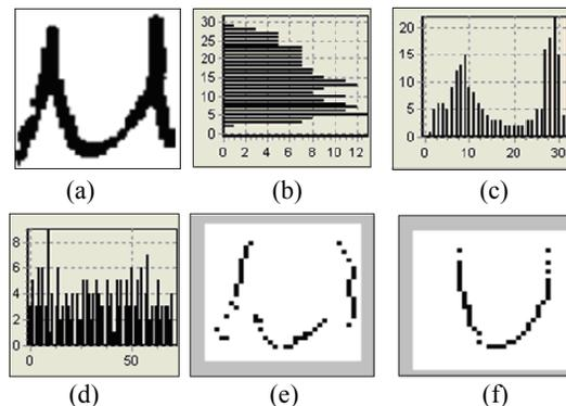
**Fig. 1: a) Character Matrix, b) Horizontal Histogram, c) Vertical Histogram d) Radial Histogram, e) Radial out-in Profile, f) Radial in-out Profile.**
