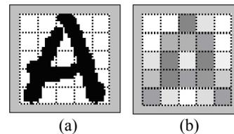
**Fig. 2: Feature extraction of a character image based on zones. (a) The normalized character image, (b) Features based on zones. Darker squares indicate higher density of character pixels.**
