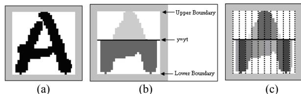
**Fig. 3: Feature extraction of a character image based on upper and lower character profile projections. (a) The normalized character image. (b) Upper and lower character profiles. (c) The extracted features. Darker squares indicate higher density of zone pixels.**
