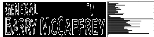
Fig. 4. Example of horizontal projection
