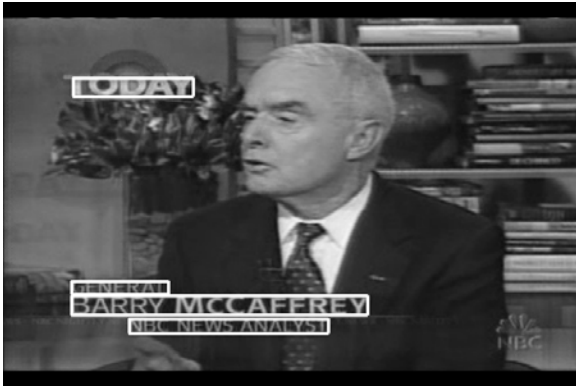
Fig. 6. Bounding boxes after projection analysis
