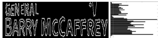
Fig. 4. Example of horizontal projection
