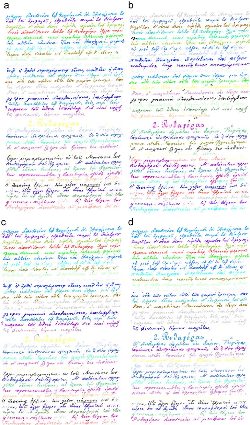
Fig. 14. Text line segmentation result on a historical document produced by (a) proposed method; (b) Hough method [4]; (c) fuzzy RLSA method [6] and (d) projection profile method [30].
