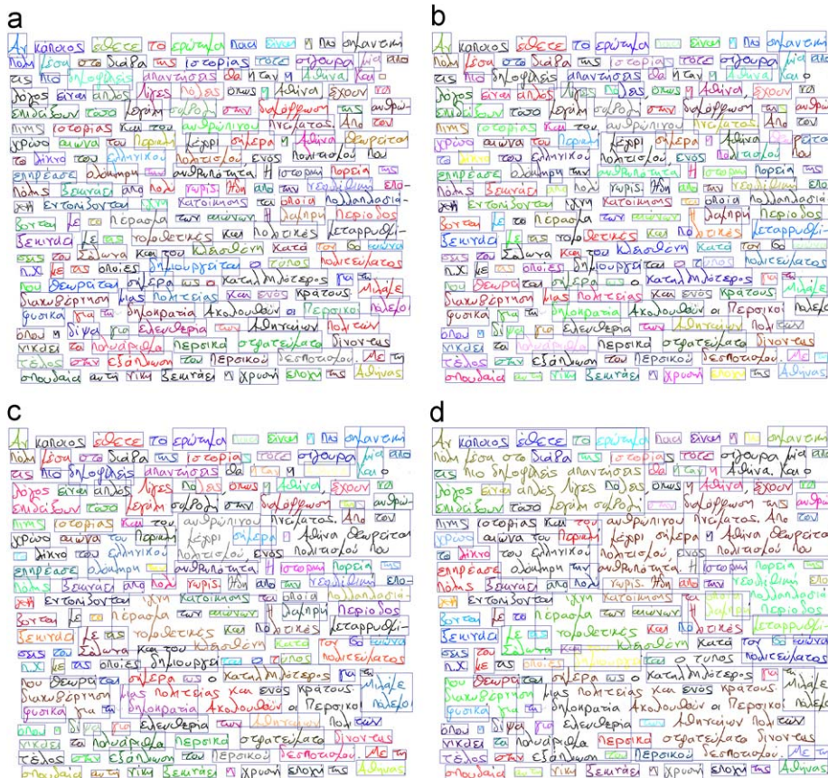
Fig. 12. Word segmentation result on Greek handwritten document when using (a) proposed methodology, (b) Hough [4] for line segmentation and RLSA [8] for word segmentation and (c) fuzzy RLSA [6] for line segmentation and RLSA [8] for word segmentation and (d) projection profile [30] for line segmentation and RLSA [8] for word segmentation.
