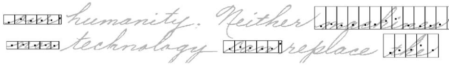
Fig. 1. An example showing the partitioning of connected components to blocks of width AW and the corresponding gravity centers. All connected components not placed in a bounding box correspond to either “Subset 2” or “Subset 3”.
