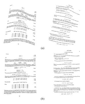
Fig. 7. Examples of coarse rectification step: (a) original document images; (b) corresponding rectified document images.
