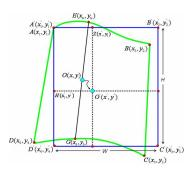
Fig. 6. Transformation model in coarse rectification:  $W = |\widehat{AB}|, H = |AD|$ and  $A'(x'_1, y'_1) \equiv A(x_1, y_1)$ .
