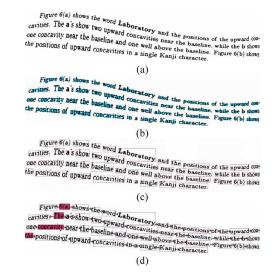
Fig. 4. Example of word and text line detection; (a) original distorted document image; (b) result after horizontal smoothing; (c) detected words; (d) detected text lines; the first word of each text line detected in the left-right and top-down scanning is indicated with a filled box and the arrows show the linked neighbor words of the same text line.
