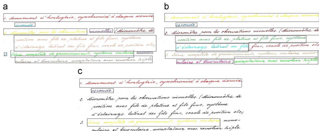
Fig. 1. An example of Step 1 in text line segmentation task; (a), (b) two different segmentation results with bounding boxes; (c) subregions from which we extract the features.
